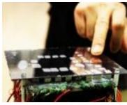
Ketsuro-Graffiti is a novel canvas that shows images with computer generated water condensation and enables users to touch them freely. Users can write or apply graffiti with their fingers on a pattern of water generated condensation. The proposed system basically consists of peltier devices, an array of heat conductive actuators, and a display surface.
